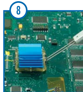
8 Using the "Forked End" of the Spring Clip tool, "latch over" the "Closed End" of the Spring Clip on to the Frame Clip tab.
